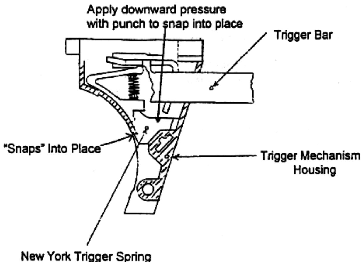
1. Detail strip the pistol frame (trigger assembly)
